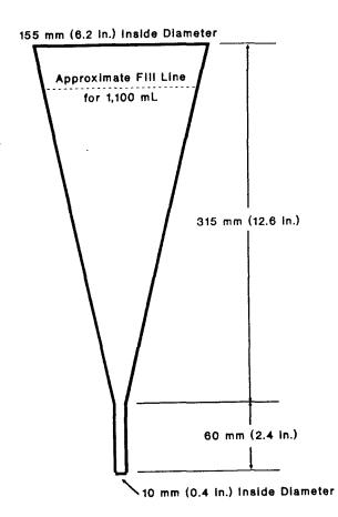
Figure 1. Cross-section of Marsh Flow Cone
